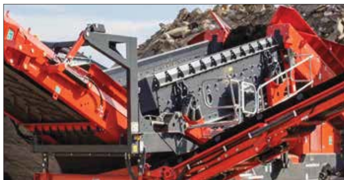
Screenbox can be Hydraulically raises to facilitate mesh changing
