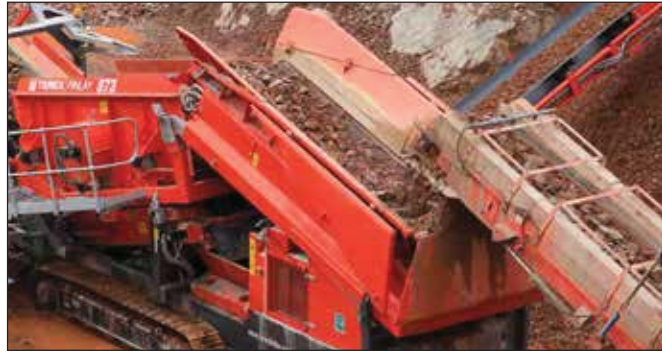
Hopper - Extensions folded for crusher feed
