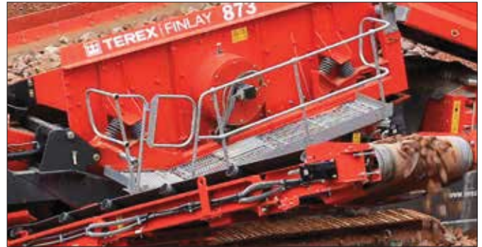
Galvanised Catwalk around Screen
